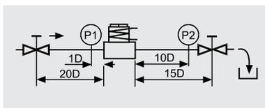
Fluid is water, specific gravity 1 kg/dm<sup>3</sup> the pressure drop P1, P2 is 1Kg/cm<sup>2</sup> in a way that the Kv is equal to the flow in liter/min.
