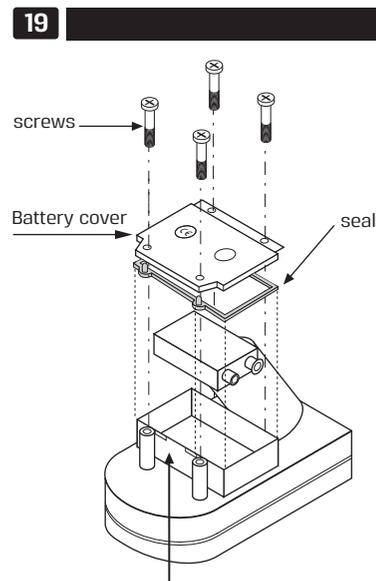
When replacing the seal, push seal tabs into slots.
